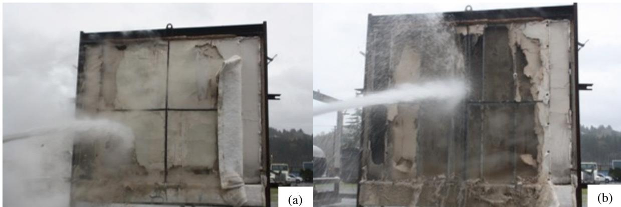
Figure 9. Test hose stream photographs showing water application near (a) the beginning and (b) the end of the test.
