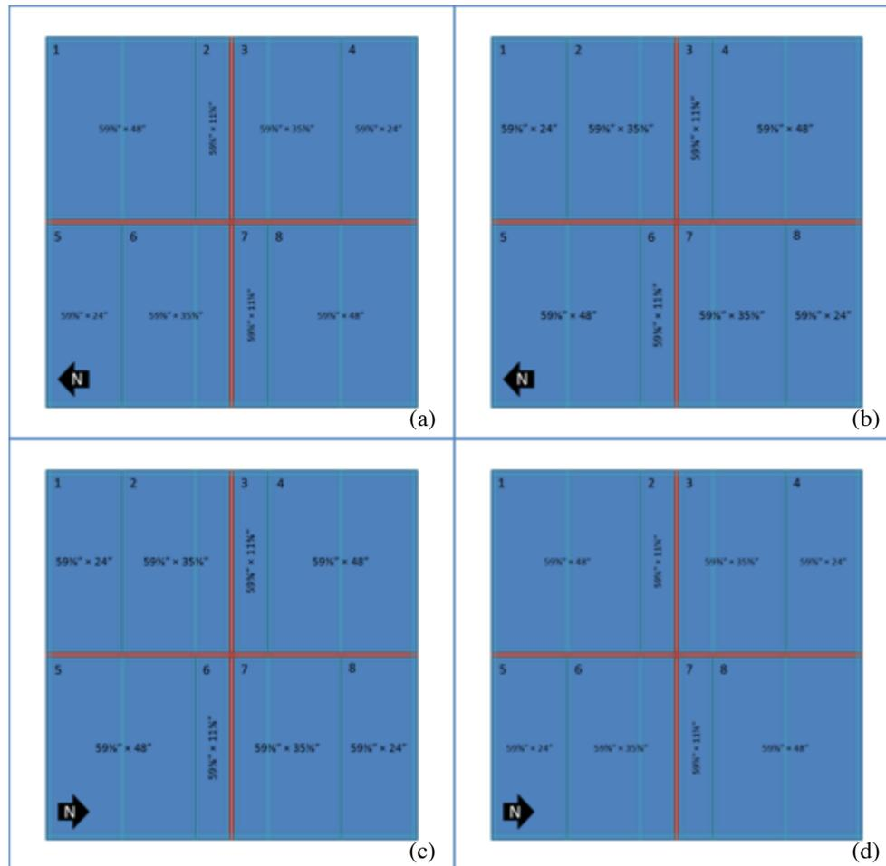
Figure 3. Schematic of drywall layout showing (a) exposed face, (b) exposed base, (c) unexposed base, and (d) unexposed face.
