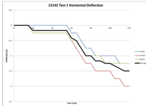
Figure 8. Horizontal deflection of wall assembly for the two-hour test exposure.
