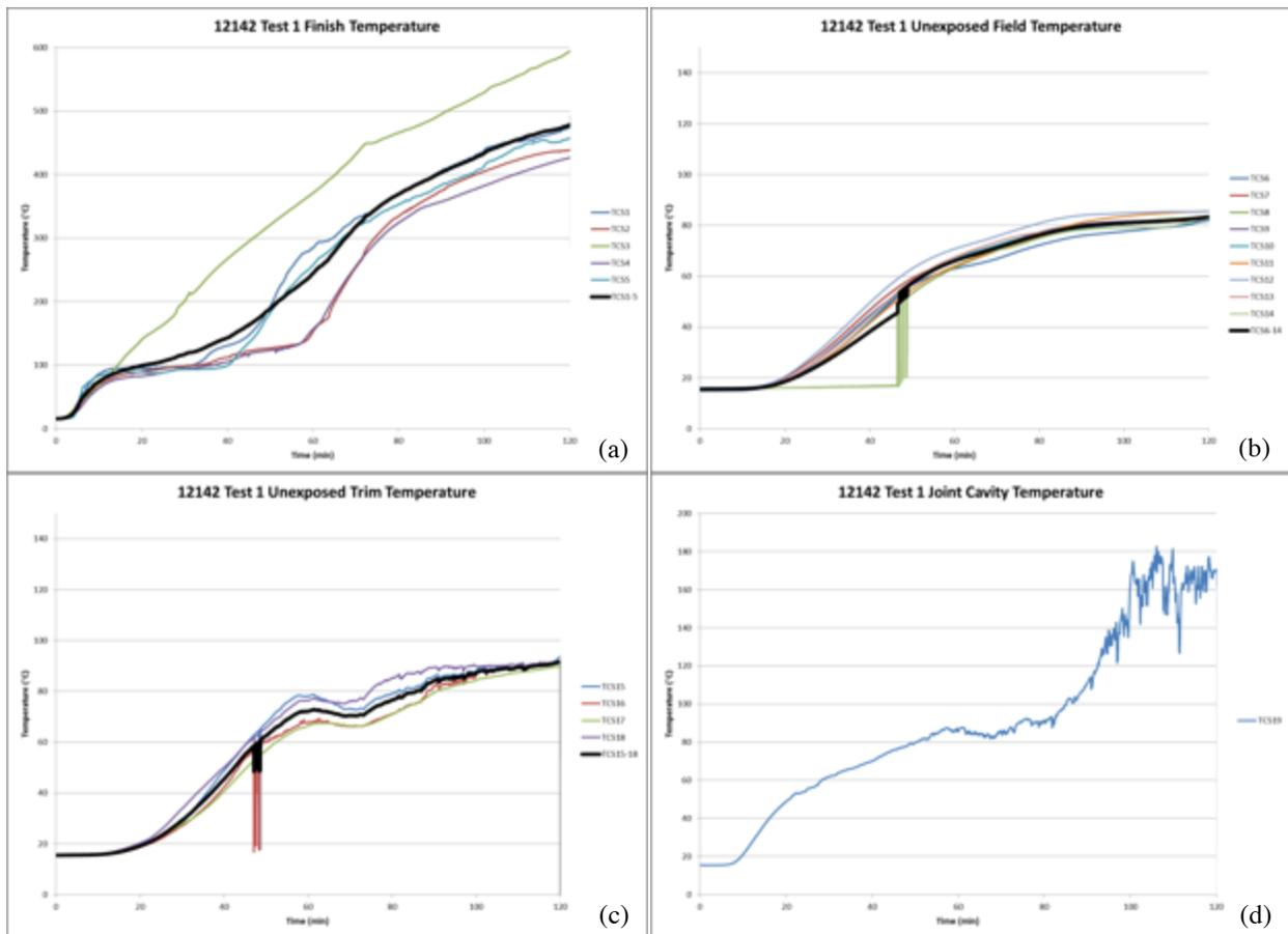
Figure 7. Sample thermocouple groups showing (a) finish TC<sub>s</sub>, (b) field TC<sub>s</sub>, (c) trim TC<sub>s</sub>, and (d) joint cavity TC<sub>s</sub>.
