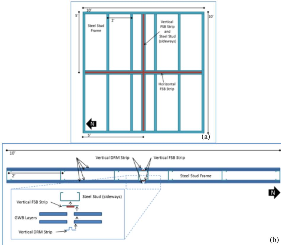
Figure 2. Schematic of wall assembly showing (a) frame, and (b) top-view cross section.
