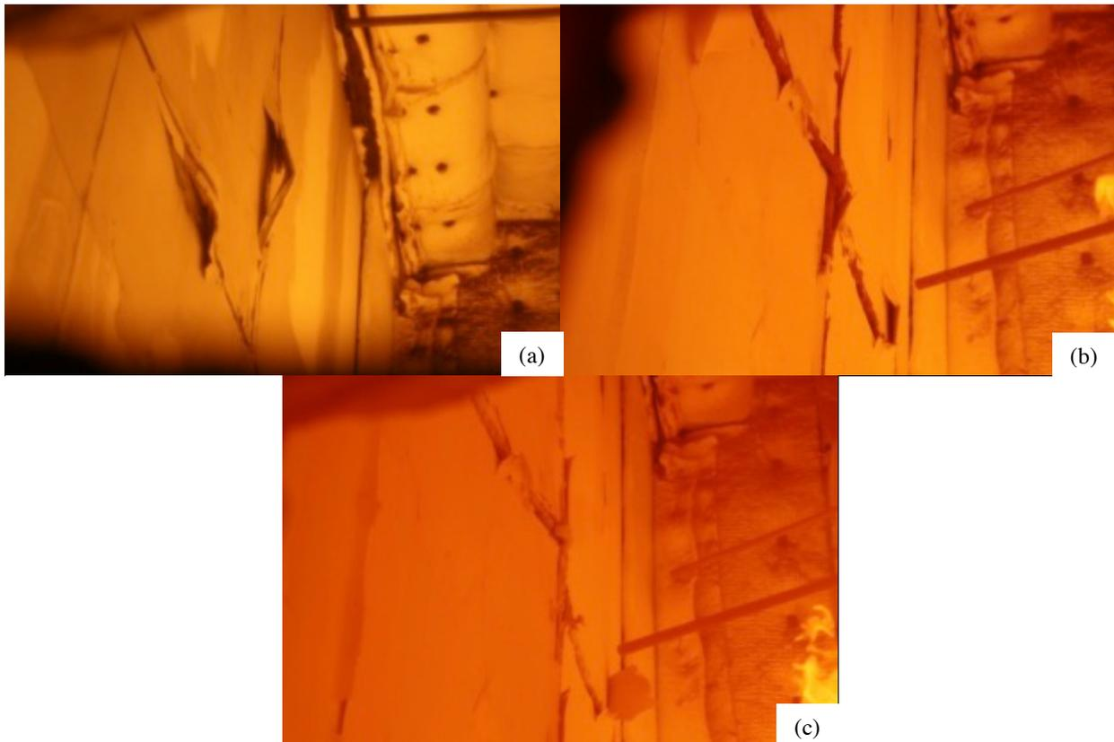
Figure 5. Test fire resistance photographs showing (a) bowing DRM trim, (b) center intumescent, (c) deteriorated center intumescent.
