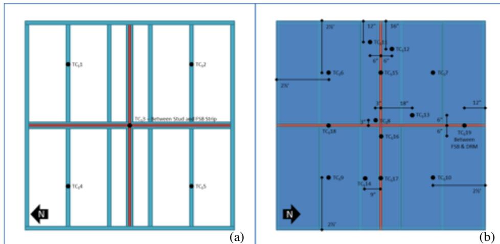
Figure 4. Sample thermocouple locations on assembly showing (a) finish TC<sub>s</sub> and (b) unexposed TC<sub>s</sub>.
