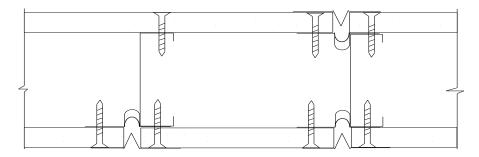
Rated 2 Hour - Top View CJB at Stud/Jamb (Single Side & Back-to-Back)
