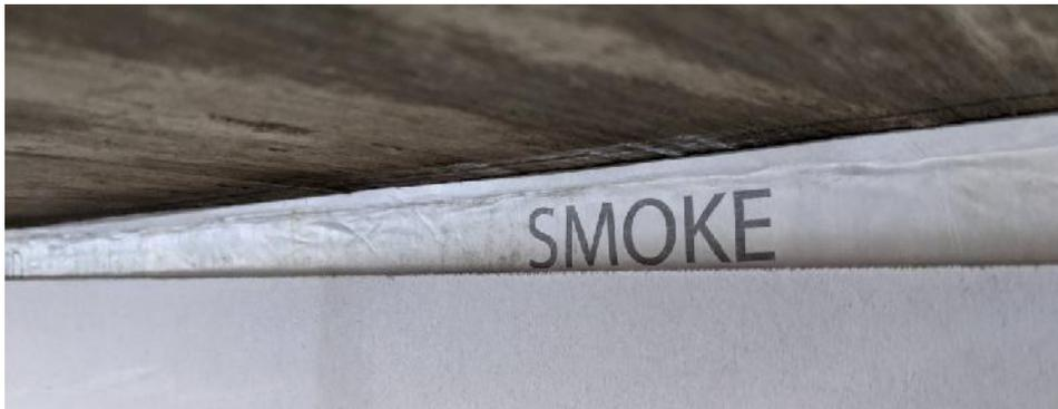
Figure 5: Minor rolling of abuse resistant coating after Class III cycling. The joint was left opened to  $3/4$  inch for air leakage testing.
