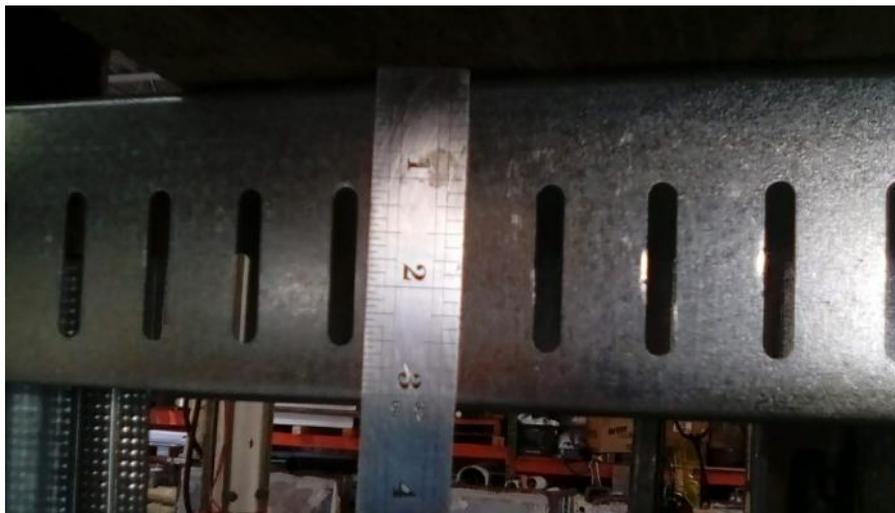
Figure 1: The top track used for the 1-hr gypsum wall assembly. The track has 1-1/2 inch long slots spaced 1 inch OC.
