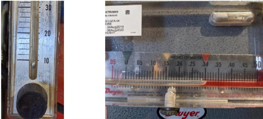
Figure 7: The air flow into the air leakage apparatus is shown on the left and the differential pressure inside the apparatus is shown on the right. This data was obtained at 400°F (elevated).
