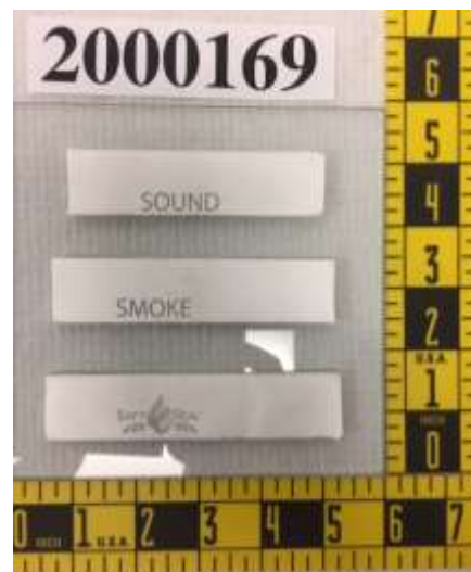
Safti-Seal™ Smoke-n-Sound “Peel and Stick” Gasket as submitted (left) and tested (right)
